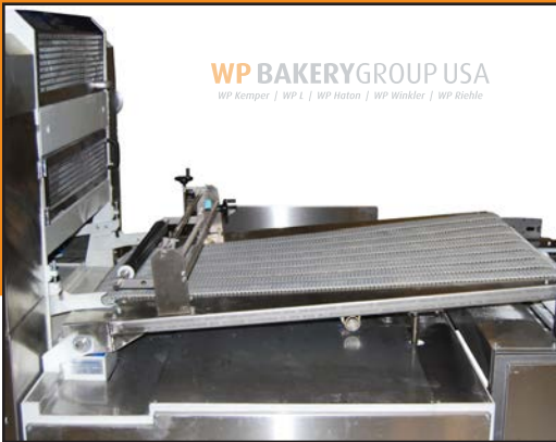
Discharge Conveyor, Steel Table & Transfer Roller
