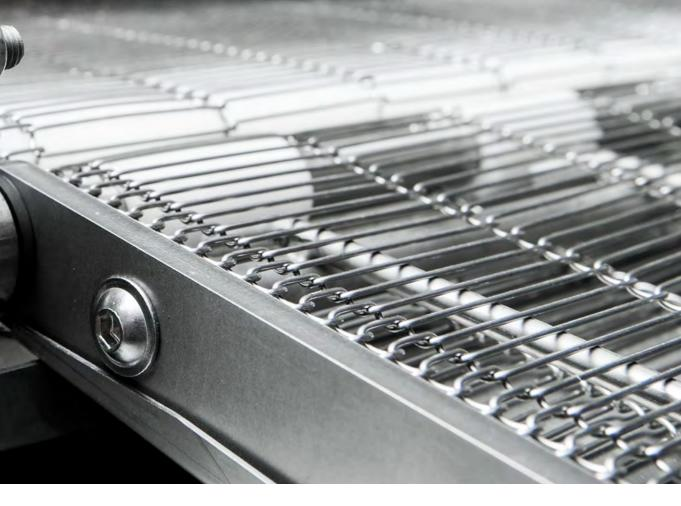
The optional salter allows for the complete baking cycle to be achieved automatically directly from the freezer. You place the products onto the stainless steel belt, push the start button and the oven does the rest. The product, in this case, is first gently thawed in the oven, exits to be salted and automatically goes back in to be finished.
