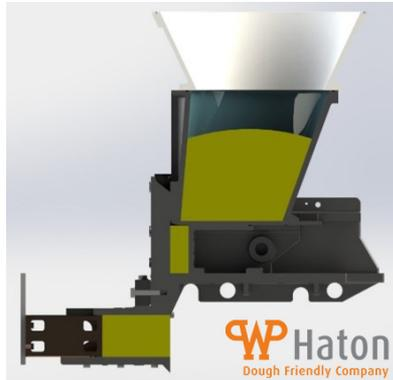
**D** the dough is ejected without pressure on the discharge conveyor while the dividing cycle is restarting again.
