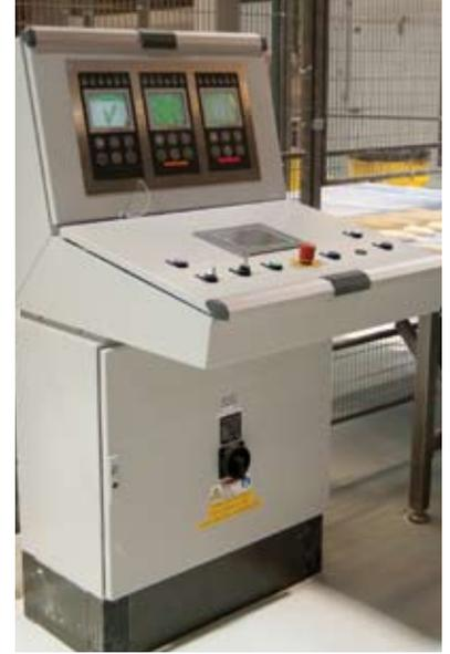
The Steward has an own control panel provided also with a display unit for the oven control and the recipe management for each oven.
