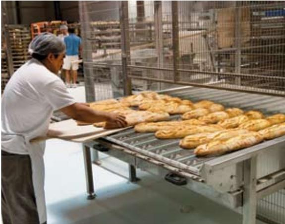
Removal of the rustic baguettes from the wire-mesh belt.
