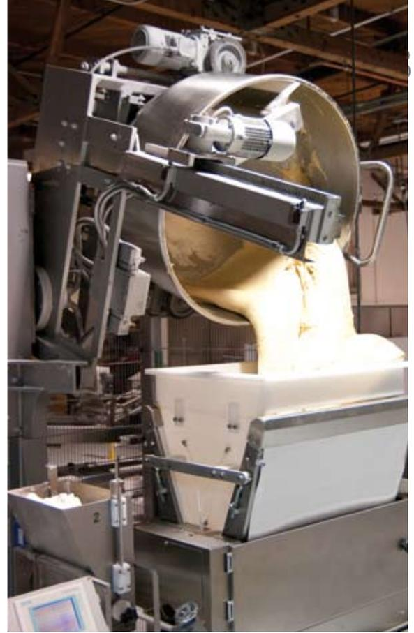
As many working steps as possible are automated. Also the dough is transported into the dough strip machine by means of a lift tipper.
