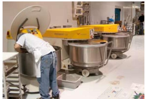
The dough is the base for the quality of the finished baked goods. For the preparation of the dough Bay Bread uses a kneader by WP Kemper.
