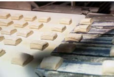
Square bread rolls. Shape and weight are determined by means of a guillotine.
