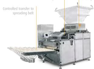
Through the use of extremely high quality construction parts and additional material reinforcement, the WP KEMPER SOFTSTAR is extremely robust. An electronic piece counter, hourly capacity display and infinitely adjustable drive are included as standard. The option of a Multi-Measuring Drum can be used, which allows the processing of multiple weight ranges.
