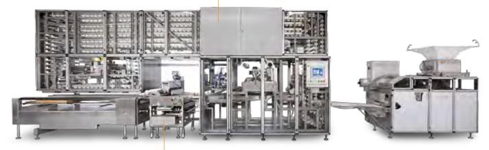
The modular design allows easy on site expansion of hourly capacity and product range. All modules can be freely combined. EVOLUTION – THE NAME OF THIS ROLL LINE CONCEPT IS IT'S PROGRAMME, IT IS THE RESPONSE TO THE CONTINUOUS
