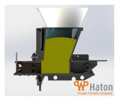
A the dough flows from the hopper in the dividing unit when the main piston moves backwards.
