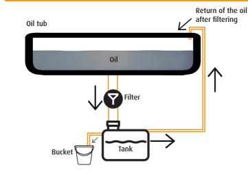
THE USED OIL IS COLLECTED IN A TANK BY THE FILTER SYSTEM AT THE END OF THE WORK AND CAN BE PUMPED BACK INTO THE OIL TUB OR DRAINED INTO A BUCKET BY THE BACKWASH PUMP AFTER THE CLEANING PROCESS HAS BEEN COMPLETED.
