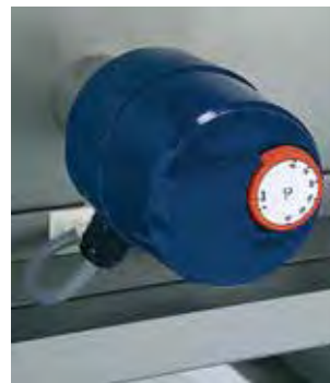
Heater for tank improves colour and shine
