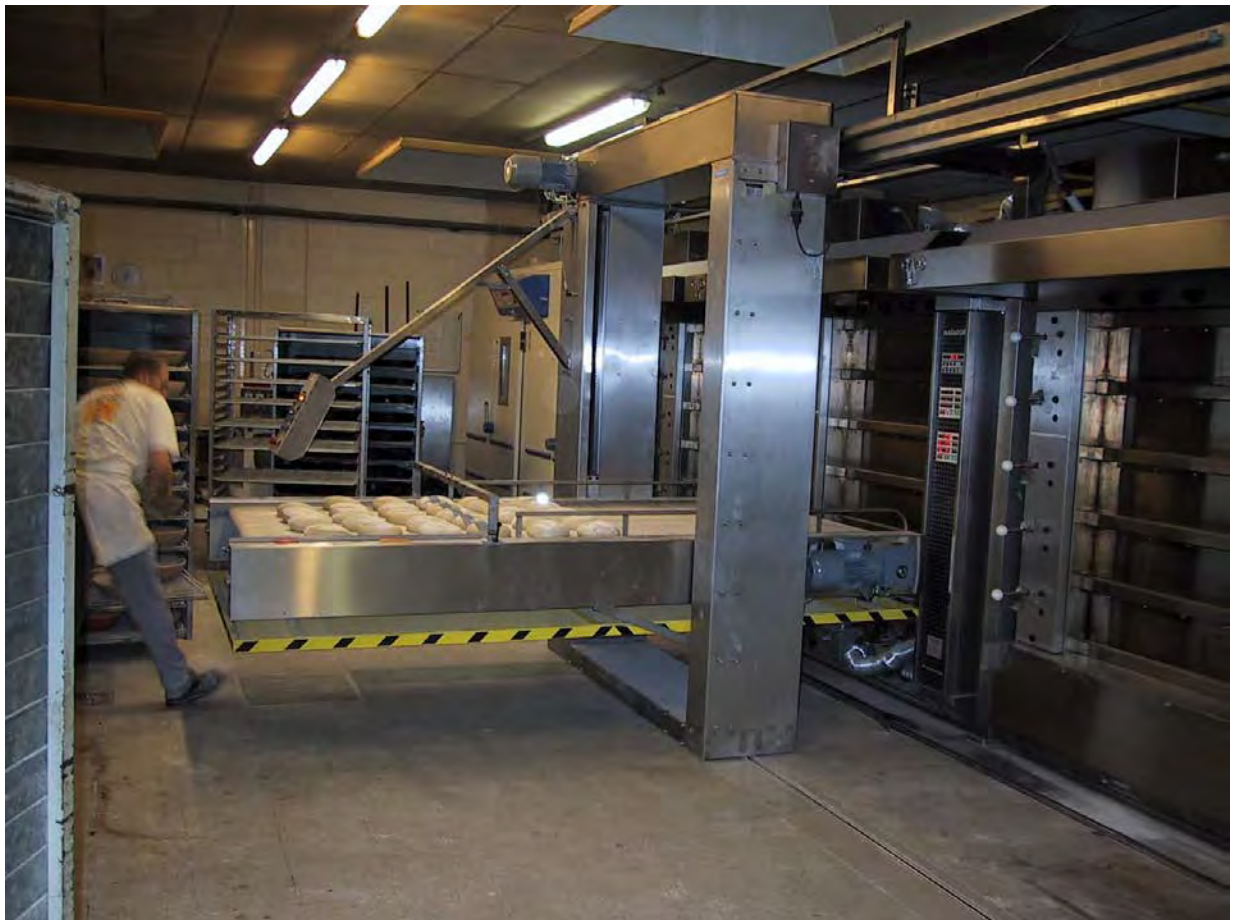
Deck oven loader LIFTMASTER with independent gear drive being loaded from an operator opposite the oven.
