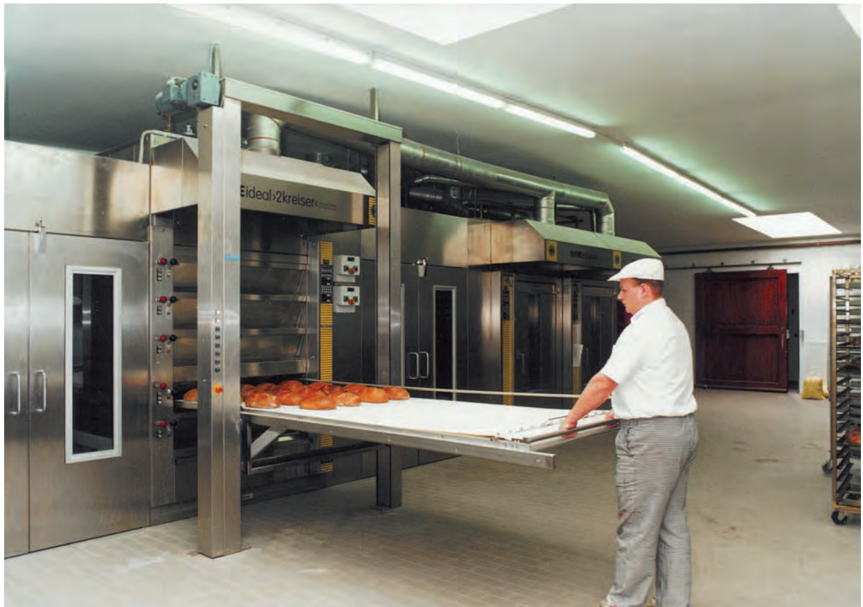
Deck oven loader LIFTMATIC with elevation drive and manually operated setter
