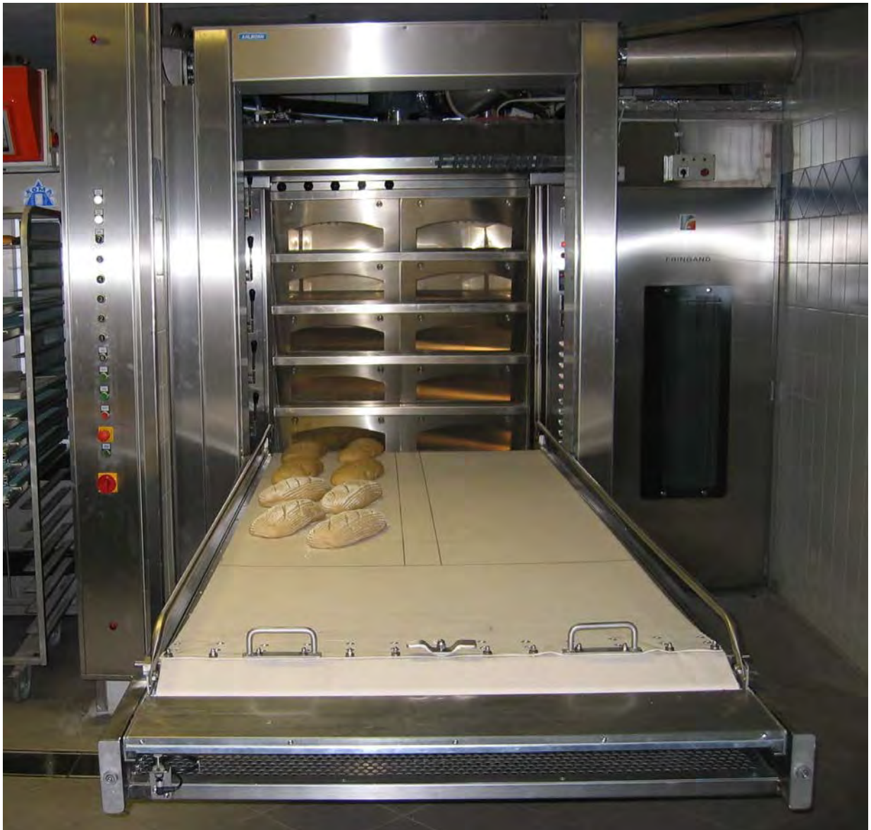
Deck oven loader LIFTMATIC S with elevation drive and motor driven setter movement
