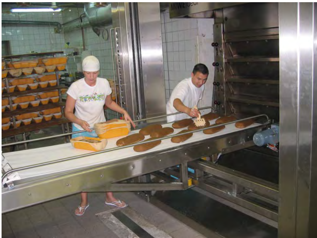
LIFTMATIC S with a 0,9m wide setter in front of a 1,8m wide oven, shown in the left (un-) loading position
