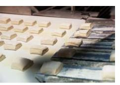
Square bread rolls. Shape and weight are determined by means of a guillotine.
